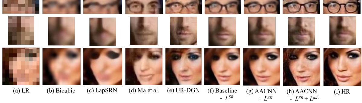
Figure 6. Comparison with the state-of-the-art methods on hallucination local test dataset. The first row is eyeglasses on "eye" part, the middle row is goatee on "mouth & nose" part, and the rest is heavy makeup on "face" part. (a) Low-resolution inputs images. (b) Bicubic interpolation. (c) LapSRN [6]. (d) Ma et al. [10]. (e) UR-DGN [16]. (f) Baseline - L^{SR} . (g) AACNN - L^{SR} . (h) AACNN- L^{SR} + L^{adv} . (i) High-resolution images. Both (g) and (h) can hallucinate specific attribute accurately in visual results. (h) is more realistic than (g) with adversarial training.
